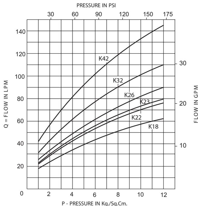
$Q = K\sqrt{P}$  where P is supply pressure in Kg/sq.cm., K= nozzle constant (K-factor) in metric
